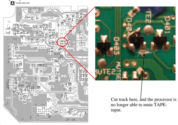
Doing this, leaves TAPE-input always active, even when playing CD or radio. To manually mute it, connect 12v to pin 7 of the TAPE input connector. Connect the 12 volts from a switch placed somewhere handy. (This requires that D404 is left in place, or that the other two tracks leading to D404 are connected.)
