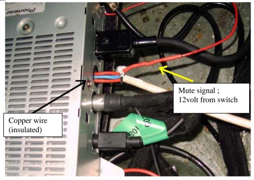
Use shielded cable only(shield is connected to ground-pin).
